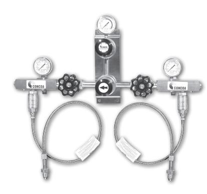
The 632 Series pressure differential switchover has been designed as a cost effective solution for high flow applications. With simple priority valve operation, the 632 delivers 15, 50, 120, or 150 psi output at flow rates exceeding 5,000 cfh. The simplistic design exceeds the stringent requirements for oxygen-acetylene NFPA 51 standards. Options include 1000watt heaters for carbon dioxide, Advantium alarms and intrinsic safety barriers for hydrogen service.
