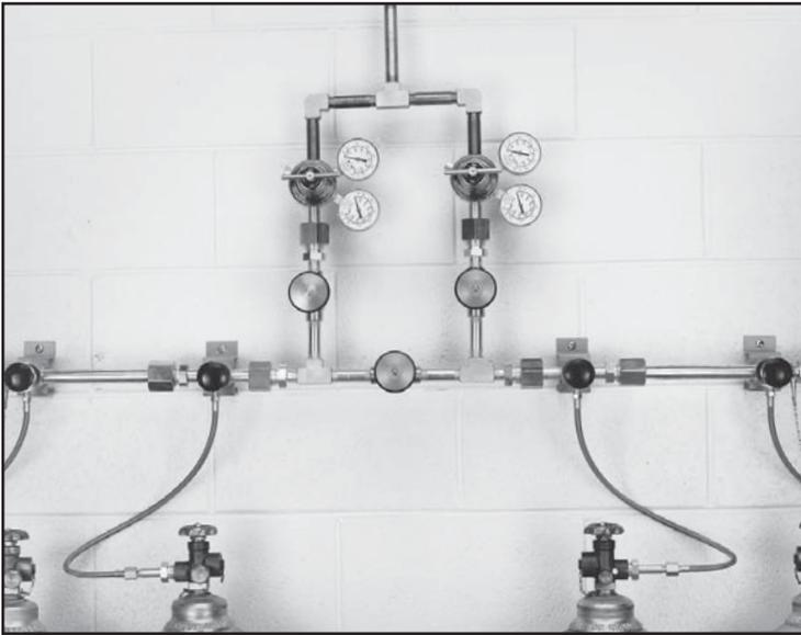
The 634 Series Switchover provides a continuous supply of gas through two extra heavy-duty 6700 Series regulators. Line or station regulators should be installed at the point of use to ensure constant delivery pressure. Use of Acetylene requires flashback arrestor on pigtails.
